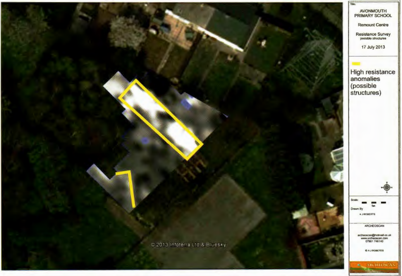
Fig. 9 Results of the Geophysical survey showing areas of high resistance in white that correspond with the location of remount depot structures.
